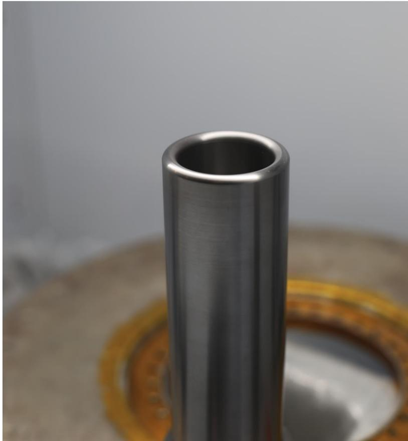
*Fig. 1 Our new beryllium anode stalk safely sitting inside a glove box, which protects us from any beryllium dust we may generate in working with the stalk. The upper opening in the part is where the plasmoid will form when the anode is in use inside FF-2B. Note the thinner wall of the new anode, which actually strengthens the part by moving the metal away from the heat source along the device axis.*
