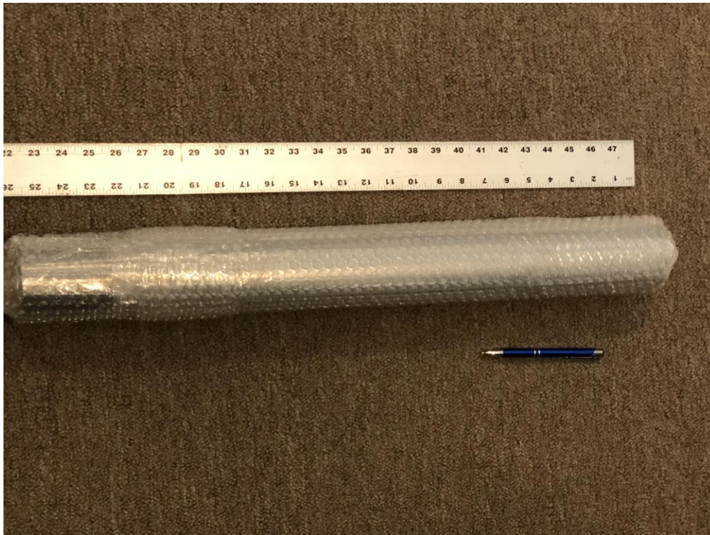
Fig 2. Our gleaming new beryllium cylinder sits safely in its plastic seal, ready to be machined into multiple anode shafts.
