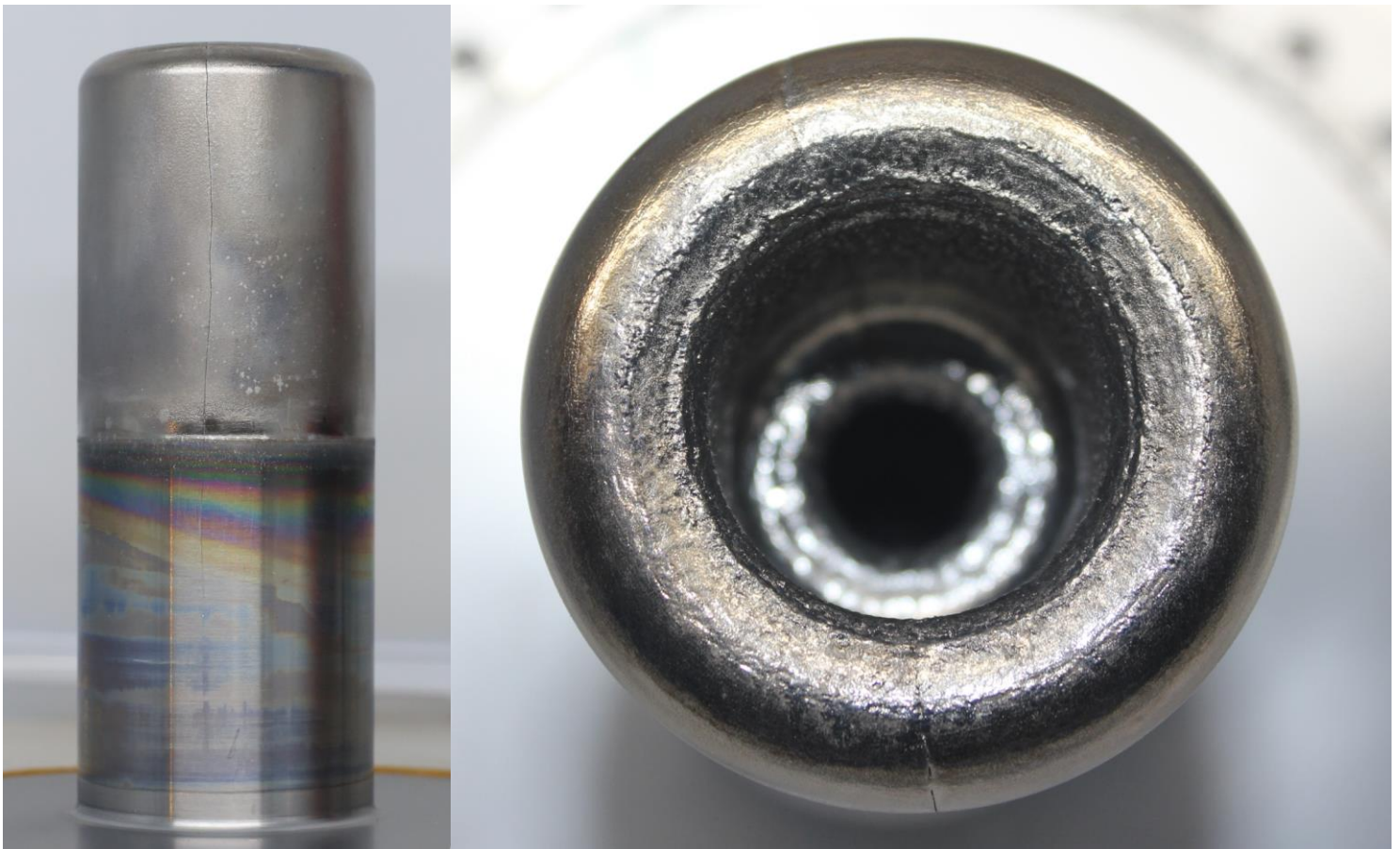
Fig. 2 Side view of anode shows one of two cracks extending down the sides. Top view shows two cracks, top and bottom extending out of the damage area on the inner lip of the anode.
