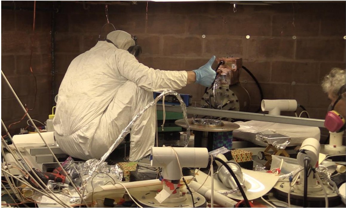
Fig. 1 LPPFusion Research Scientist Dr. Syed Hassan, fully protected against any release of beryllium dust, signals to Chief Scientist Eric Lerner the successful removal of the cracked anode (dimly visible under steel plate attached to steel beam).
