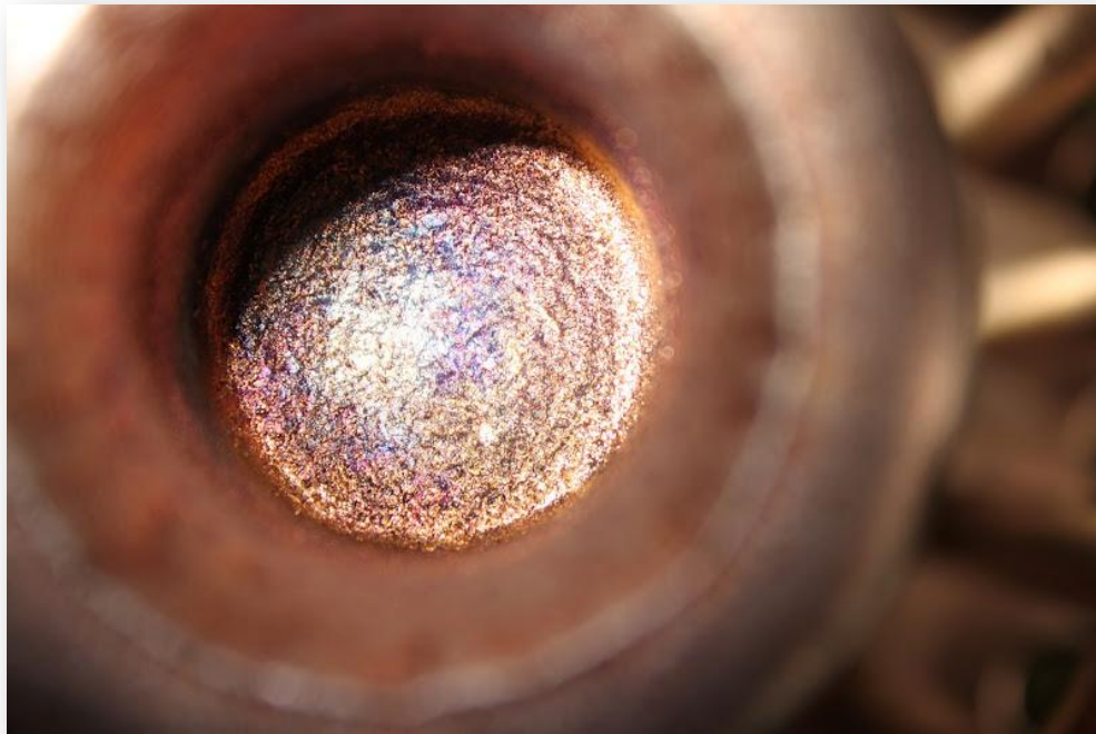
The interior of FF-1's anode, etched by the electron beams of hundreds of fusion shots... with many more on the way!
