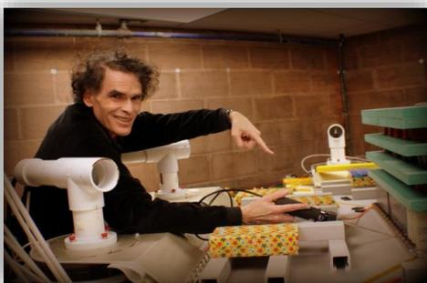
*At left: Eric points with some relief to the area showing high helium concentration, indicating the pathway to the location of our soon-to-be-fixed leak. In his right hand he is holding the needle probe of the helium detector.*
