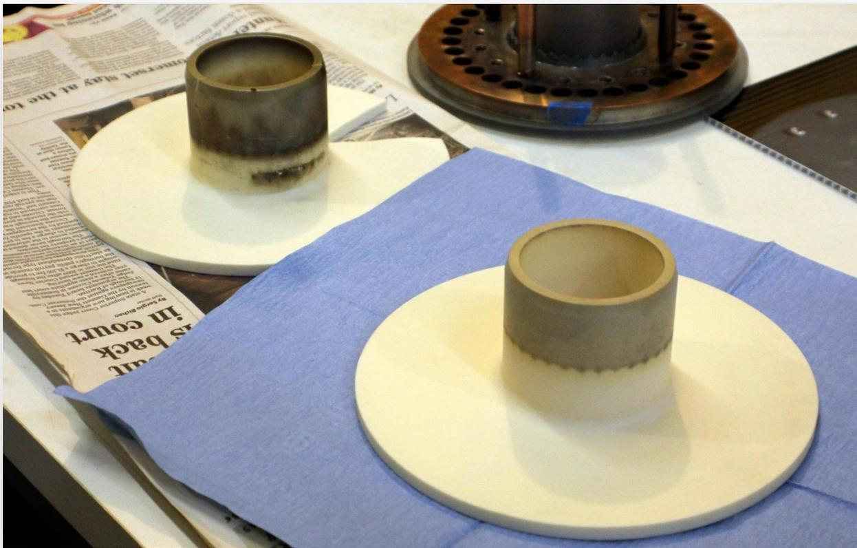
*Above: The previous, now broken insulator (background) shows arcing, with a dark horizontal mark below where the insulator should be exposed to plasma. In the foreground, the most recent insulator is pristine below the sawteeth where the plasma sheath forms.*
