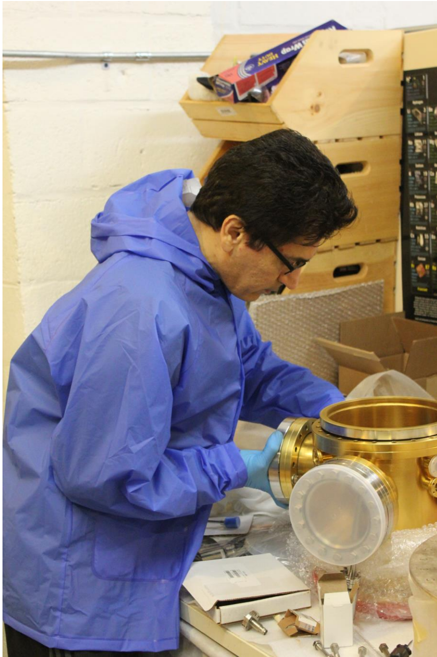
Figure 1. Dr. Syed Hassan bolts a window to the new vacuum chamber, which is coated with golden-colored titanium nitride. The protective shutter has already been installed on a second window, facing the viewer. Note the small silver lever extending below the window, which can open and close the shutter without breaking the vacuum. This window is protected by a plastic cover during assembly.
