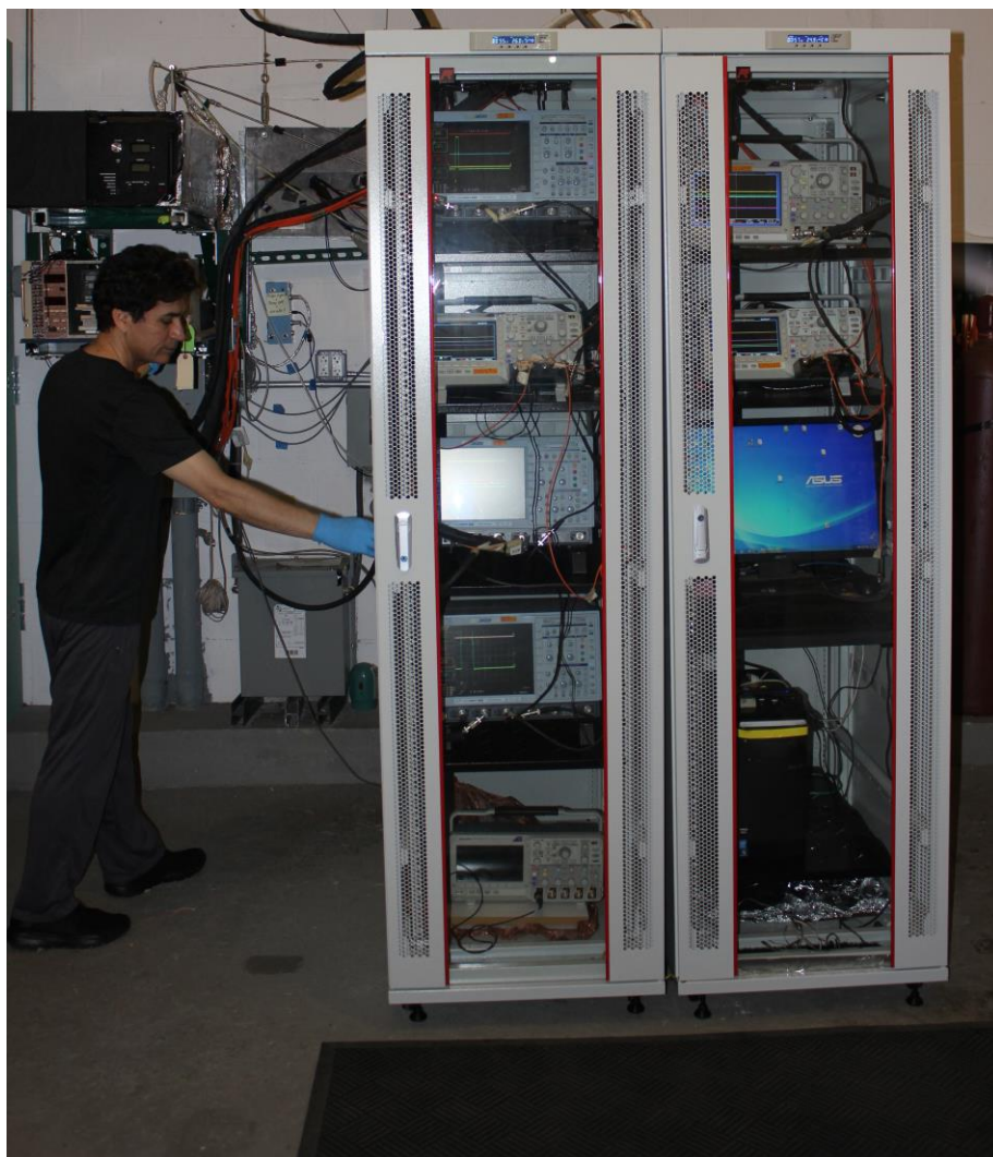
Figure 1. Dr. Syed Hassan presses the trigger button to test connections on the newly-installed Faraday cage protecting the oscilloscopes, data computer and several instruments.
