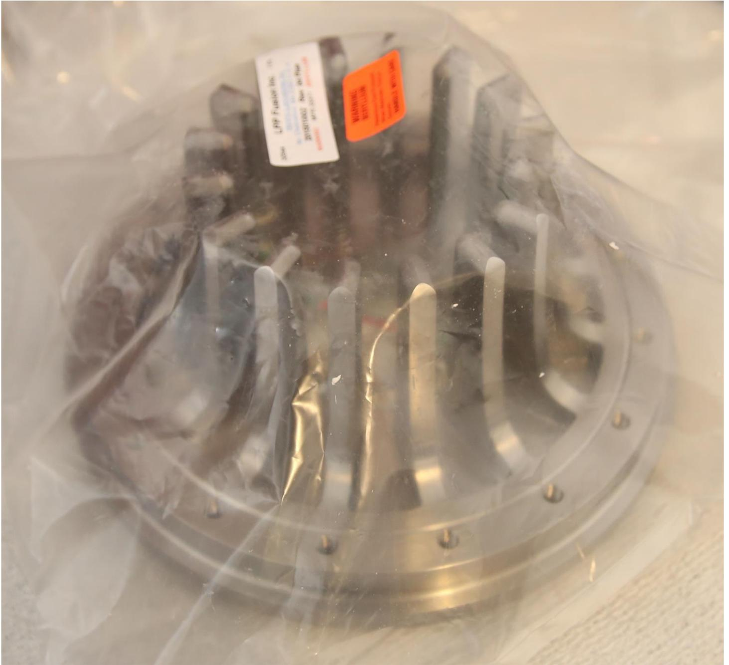
*Figure 1. The new beryllium cathode (25 cm or 10 inches in diameter) sits at LPPFusion's lab in its sealed bag. The protection is needed because exposure to atmospheric humidity for too long can damage the part's surface.*
