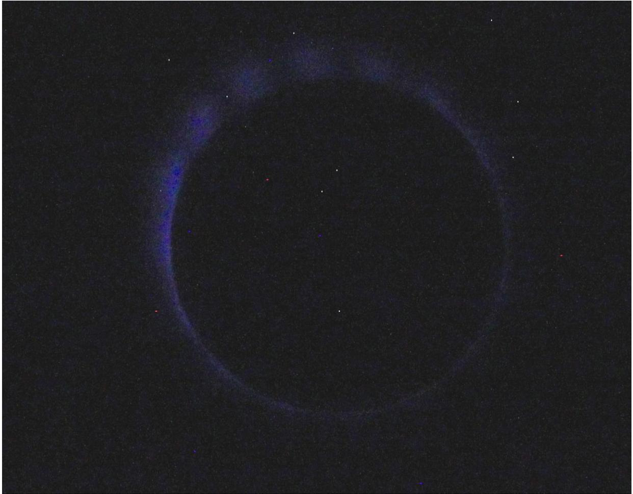
*Fig. 1. Looks like a total solar eclipse, but it's not! This is a photo of the ghostly glow of preionization from the end of our tungsten anode. The anode is the black circle in the middle and the "corona discharge" from a tiny current is creating the violet glow around the anode. When we fire the machine, these ionized regions will smooth the path of the million-amp current, reducing vaporization from the anode and thus impurities in the plasma.*
