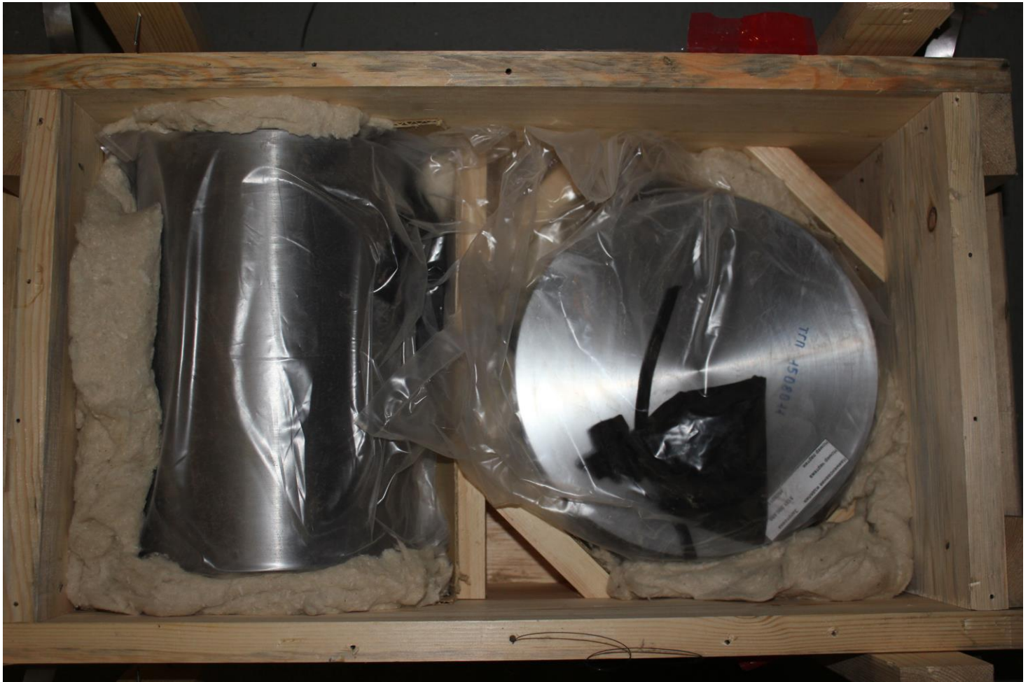
Figure 1. The new beryllium cylinders in their sturdy packing box at LPPFusion's Middlesex, NJ lab. The one on the left will go to making two anodes, of different lengths, and the one on the right will go to making a single cathode.
