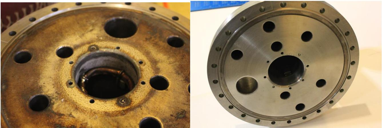
*Fig. 1 The bottom of the vacuum chamber (which is also the top of the drift tube, attached at central hole) was eroded by ions beams and heavily coated with tungsten bronze after shots in September (left). After extensive lathing and polishing, the part is almost pristine and ready to be coated with titanium nitride (right).*
