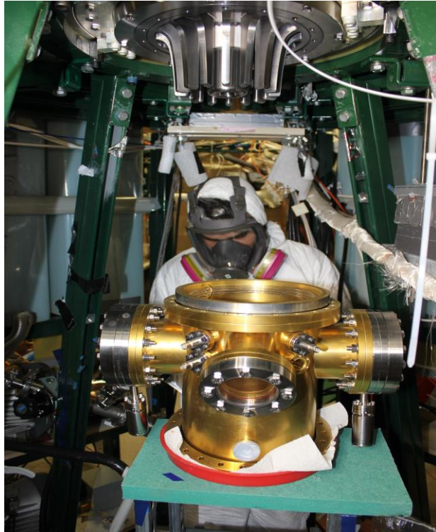
Figure 8. Dr. Hassan, in full protective dress, prepares to install the new vacuum chamber onto the beryllium electrodes, which are already attached to the device. The gold color of the chamber is from its titanium nitride coating, which prevents oxygen from escaping the underlying stainless steel.
