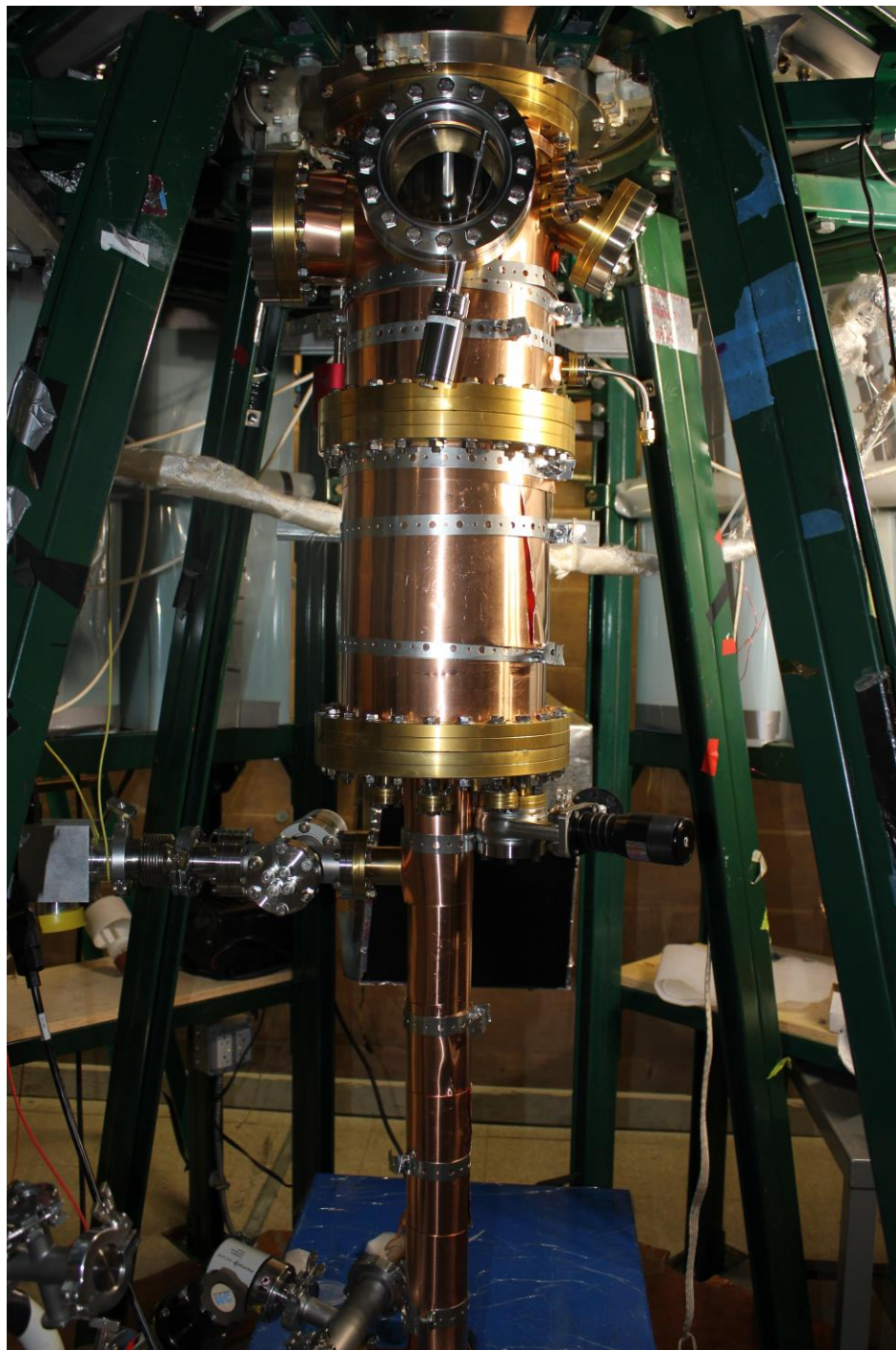
Figure 10. The vacuum chamber and drift tube (thin tube below) get copper sheet cladding to spread the heat out evenly during bake-out.
