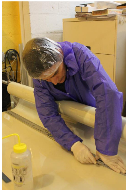
Fig. 2 Dr. Syed Hassan demonstrates some extraordinary ability in cutting Mylar to replace damaged pieces. Cutting precision will help insure no currents can arc through the gaps between Mylar pieces.
