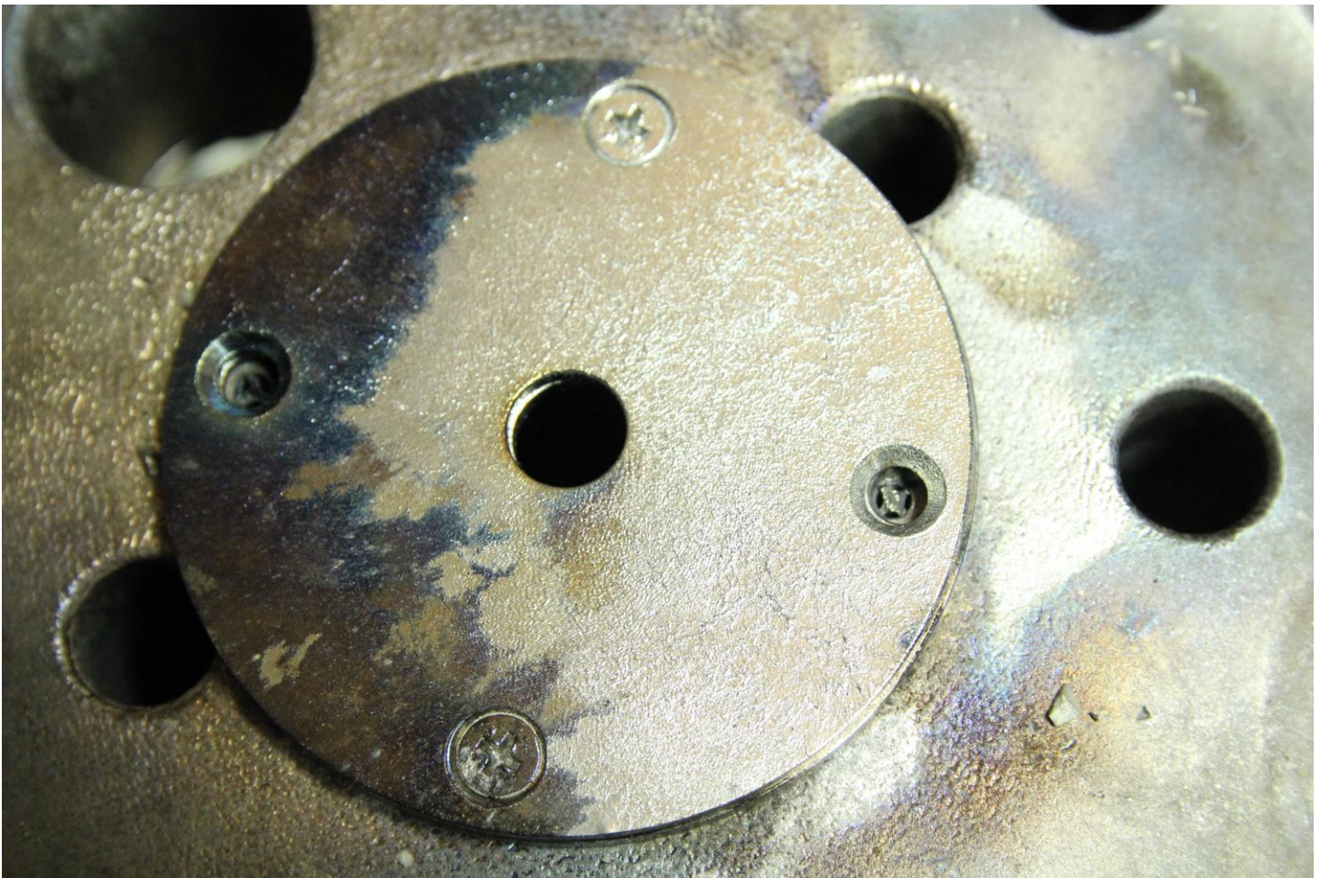
Figure 1. Tungsten bronze deposits are seen here on the steel plate at the bottom of the vacuum chamber. The small central hole leads to the drift tube, where the ions beam is measured.
