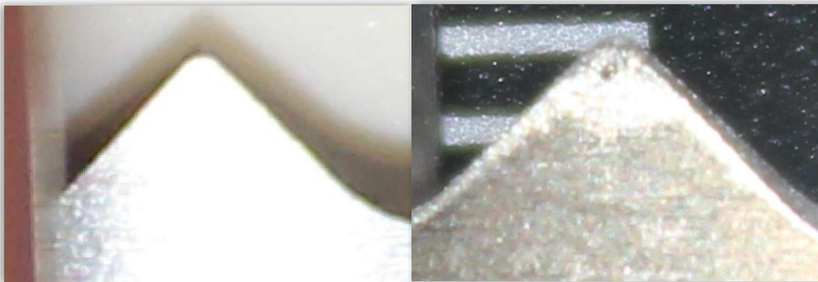
Figure 1: At left, a tungsten tooth in November, 2012; at right, a tooth in October 13, 2013
