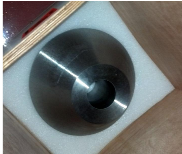
The tungsten blank, with outer diameter of 12" and total weight approaching 200 lbs, is prepped for shipping from San Diego.
