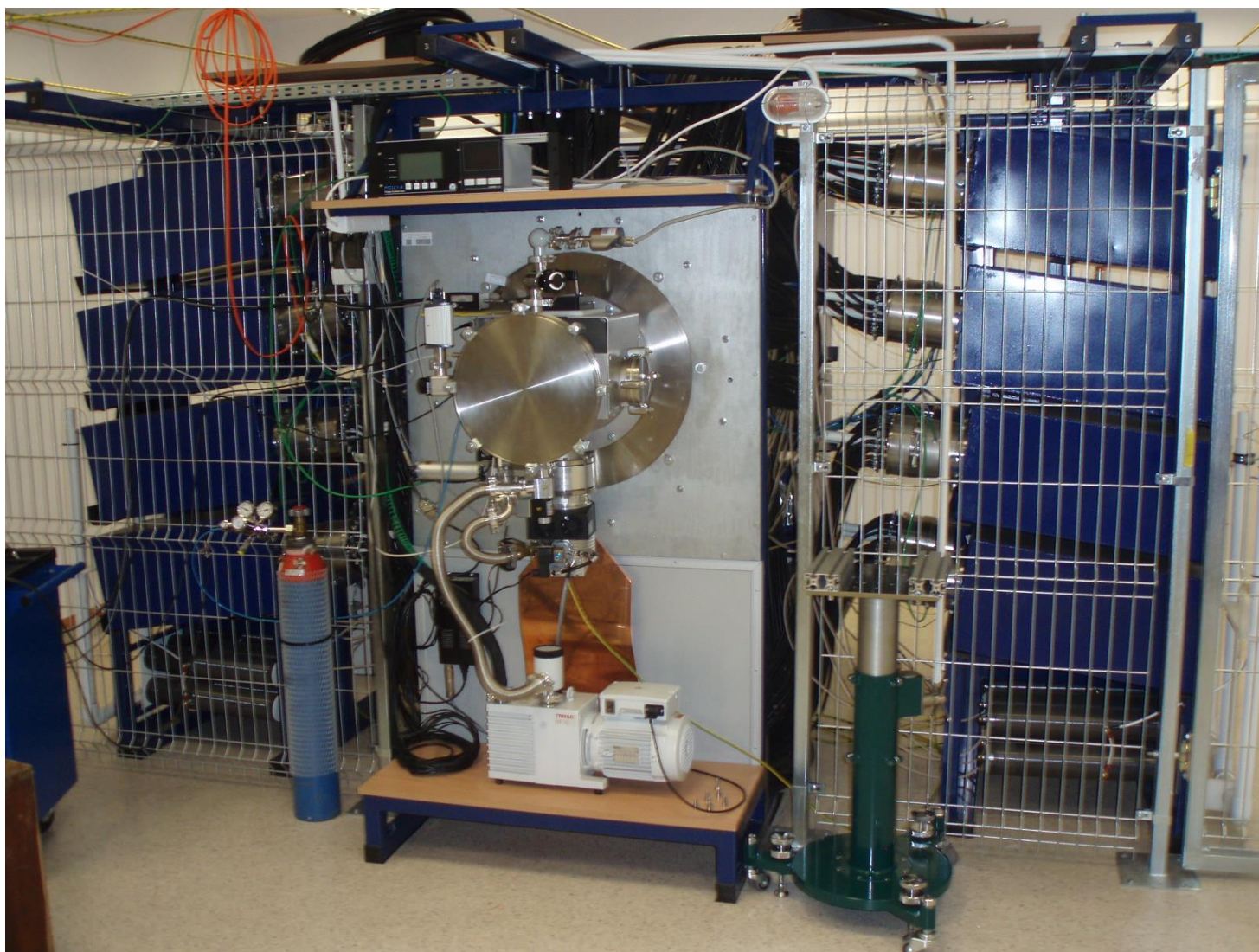
Figure 4. Institute of Nuclear Physics PF-24 plasma focus device in Krakow. The blue boxes are 24 capacitors, providing current to the electrodes inside the steel vacuum chamber (center).
