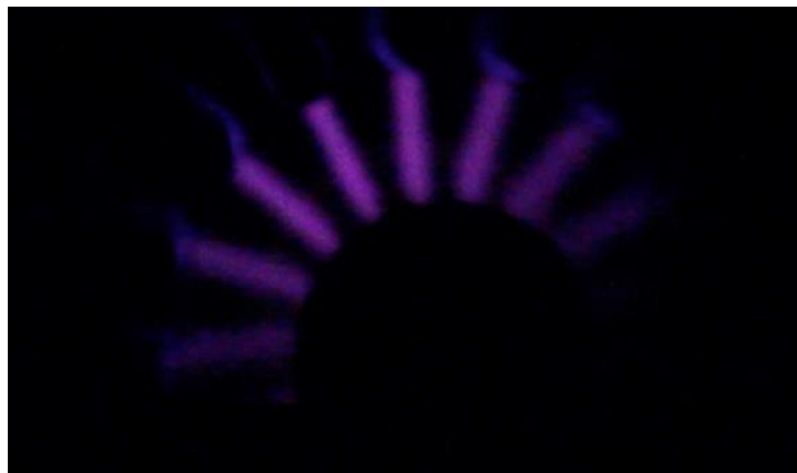
Fig. 2 A preionization pulse lights up the plasma between the tungsten cathode (outer circle) and anode (inner circle). Each glowing line connects with one cathode vane. From this window about half of the 16 vanes are visible. The left- and right-most discharges appear dimmer only because of the perspective of the camera.
