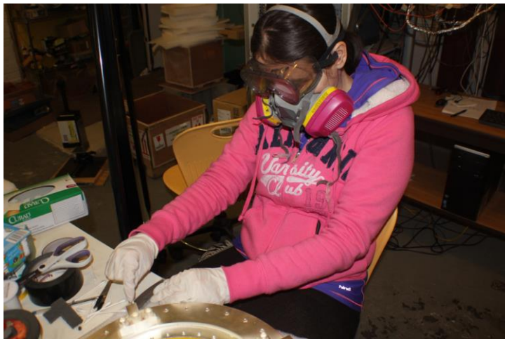
Figure 2. LPPF CIO Karamitsos cleans a scrap piece of tungsten with acetone and ammonia to decrease resistance in another test. The silver-plated steel ring at bottom will attach to the tungsten anode and deliver current to it.
