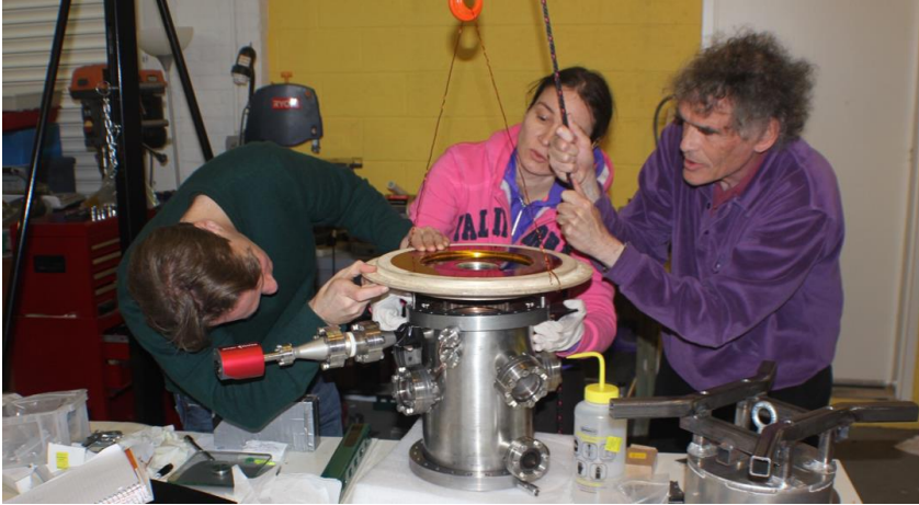
Figure 1. In preparation for assembly of the tungsten electrode onto FF-1, LPPF team members (Left to right) John Harhai, Ivy Karamitsos and Eric Lerner assemble the old cathode onto the vacuum chamber for a test of the compression of the sealing O-ring.
