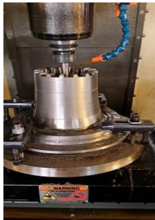
Fig 1- Tungsten cathode undergoing machining in China on Nov 19, two weeks into the two-month long process. Note the 16 vanes emerging from the tungsten blank. The inward-facing surfaces of the vanes will carry the current once the finished piece is in FF-1.
