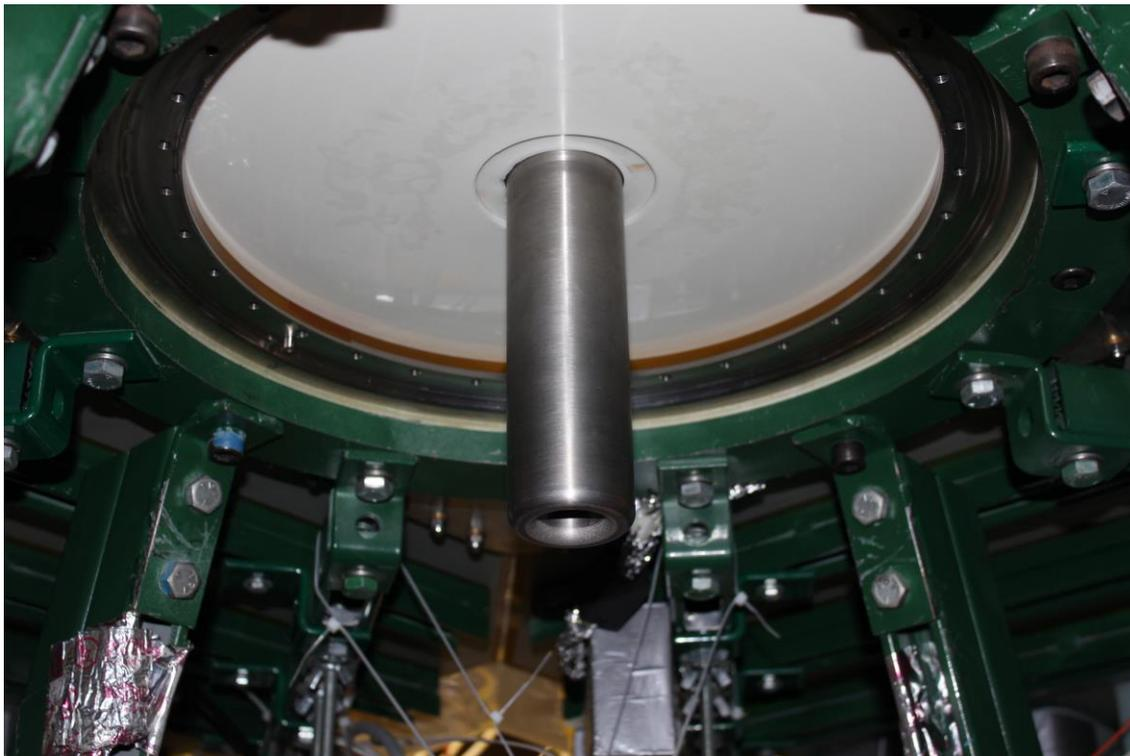
*Figure 1. The new monolithic tungsten anode rests inside FF-1. Its base is surrounded by the insulating layers of Mylar that will keep the current from shorting out to the cathode, to be mounted below it.*
