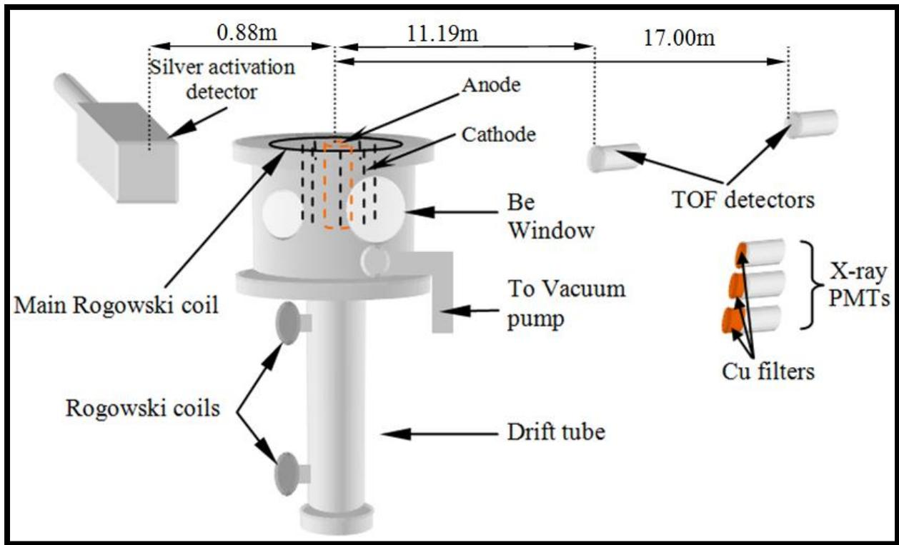
Figure 1. Experimental setup of Focus Fusion-1
