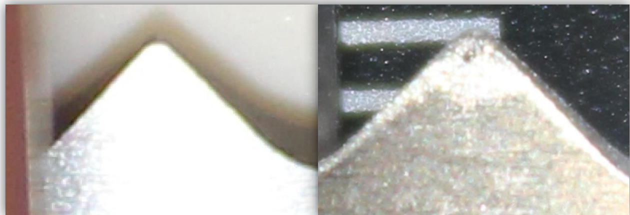
Figure 1: At left, a tungsten tooth in November, 2012; at right, a tooth in October 2013
